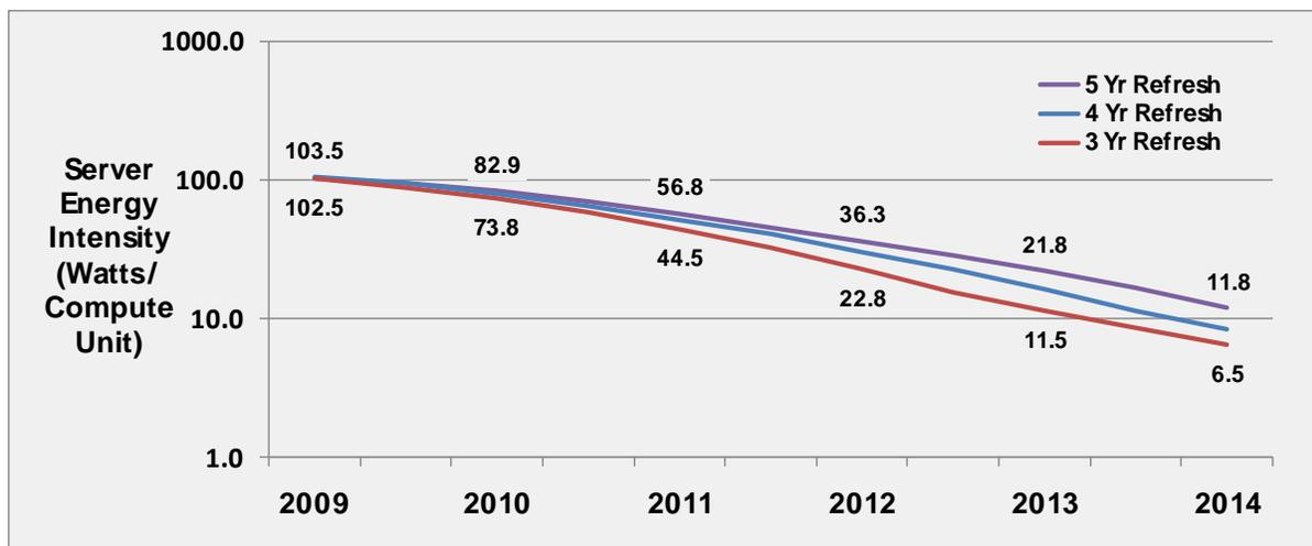
**Figure 6. Server Energy Intensity as a Function of Hardware Refresh Rate**
