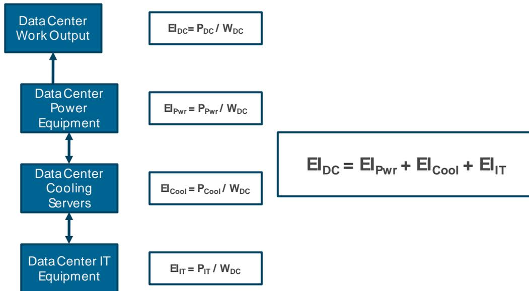
**Figure 1. Basic Data Center Energy Intensity Decomposition**
