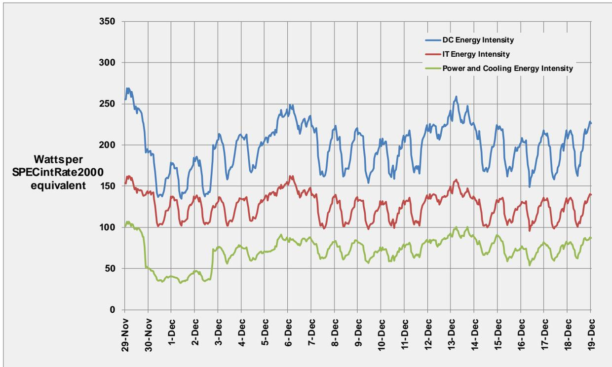
**Figure 4. Data Center and Component Energy Intensity Over a Three-Week Period**
