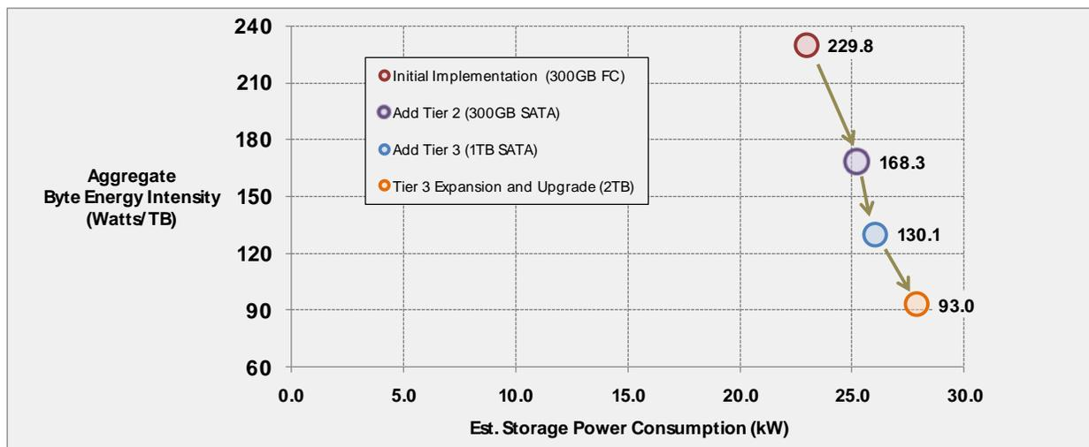
**Figure 9. Changes in Energy Intensity and Power Consumption Through Tiered Storage**
