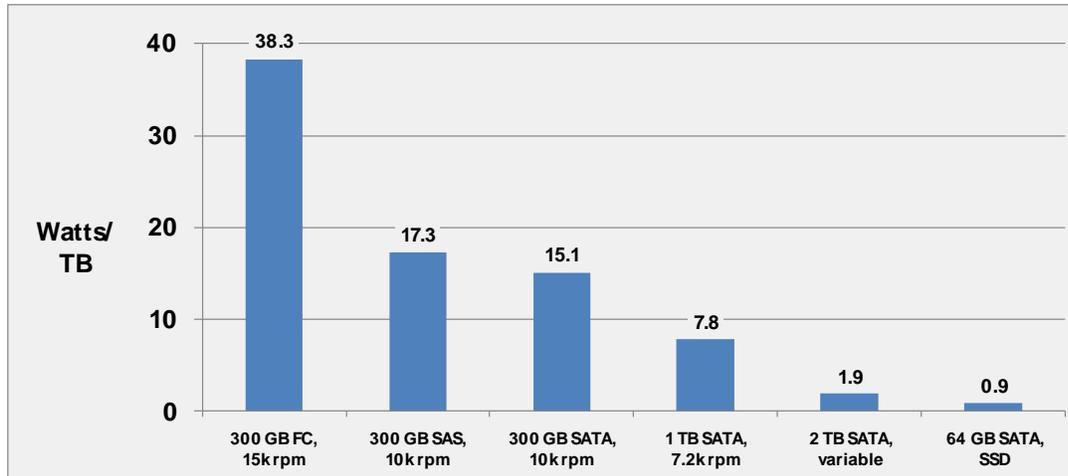
Figure 7. Minimum Storage Energy Intensity for Selected Enterprise Hard Drives<sup>8</sup>
