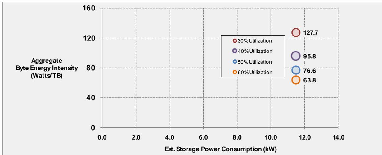
Figure 10. Effect of Utilization on Storage Energy Intensity
